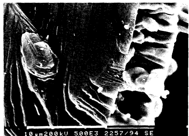
Fig. 6. High frequency sputtered ZrO 2 layer (4 h) on single crystal \alpha -Al 2 O 3 fibre, after reaction bonding at 1500°C.
