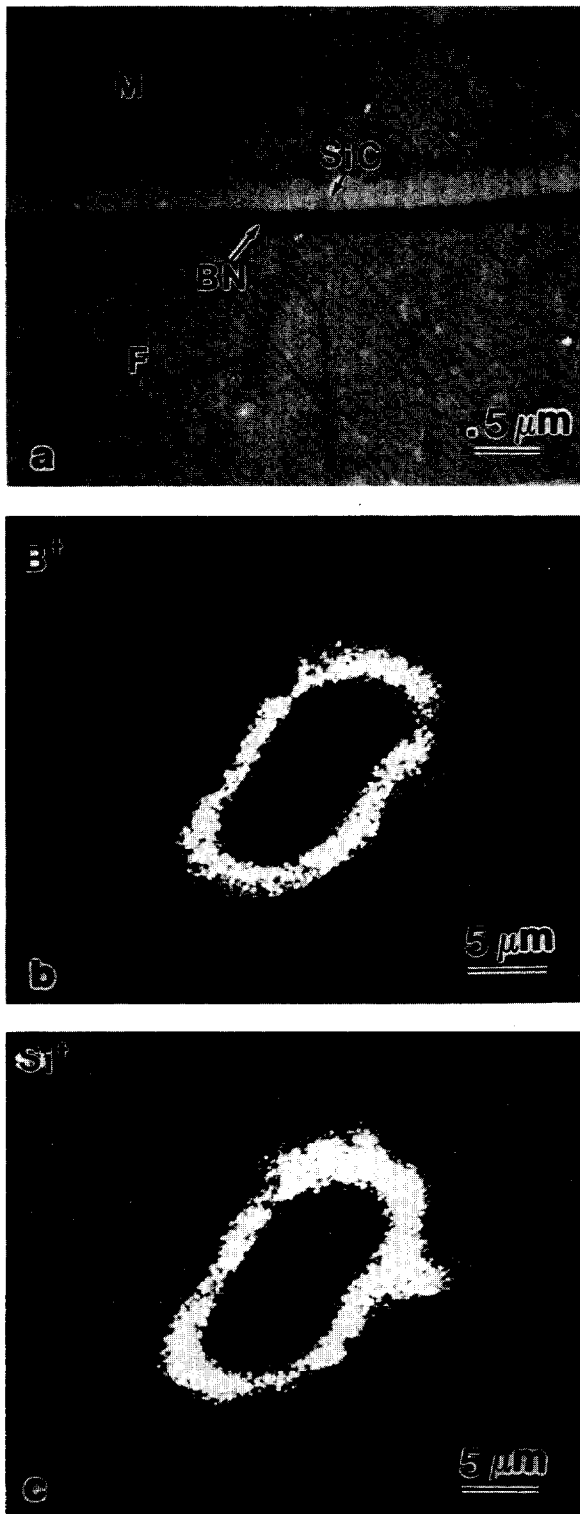
Fig. 3. (a) Cross-section of a SiC/BN coating Nextel 550 fiber, showing the double coating, (M: matrix, F: fiber); (b and c) SIMS analysis of the surface of a SiC/BN-coated Nextel 550/mullite composite, showing the presence of boron and silicon.
