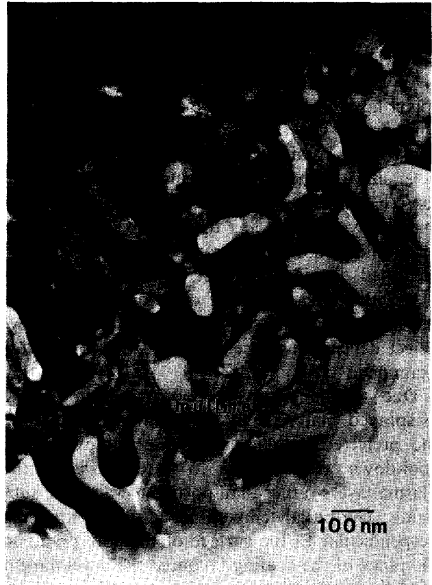
Fig. 5. Early stages in development of dendritic grain morphology in the mullite layer. Note the high density of intra-granular porosity.
