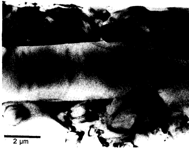
Fig. 6. Micrograph (TEM) of Nextel 440 fibres heat-treated at 1600°C, 4 h: secondary grain growth of mullite.
