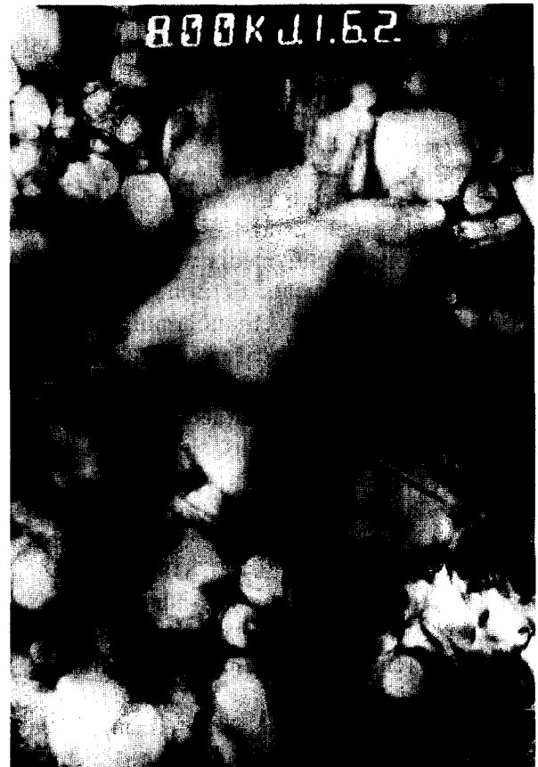
Fig. 5. Transmission electron micrograph of sample 1, for material sintered with C in Ar at 1900°C, showing rounded grains. The length of the bar is 3.1 \mu\text{m} .
