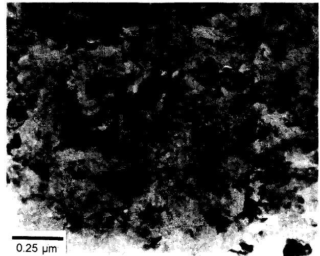
Fig. 4. Micrograph (TEM) of Nextel 440 fibres heat-treated at 1200^\circ\text{C} , 4 h: irregular-shaped mullite grains.
