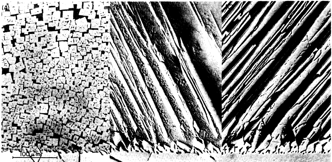
Fig. 3. Microstructures of diffusion zones in couples of sapphire (bottom) and fused silica annealed at 1900°C for 15 min and (A) quenched, (B) cooled at a relatively moderate rate and (C) cooled relatively slowly. Precipitates in diffusion zone in (A) are mullite (light grey), in (B) alumina (light grey needles) and mullite (fine precipitates between alumina needles) and in (C) alumina (light grey needles; precipitates along interface in (B) and (C) are also alumina).
