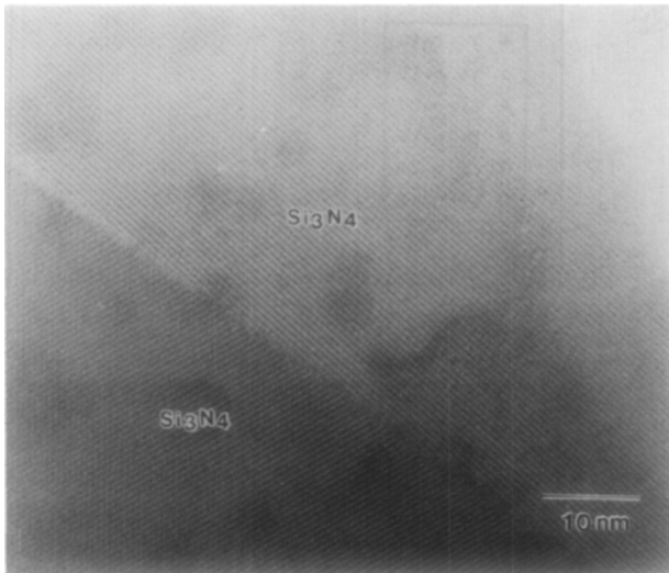
Fig. 18. Lattice imaging showing a rare case of a glass-free \text{Si}_3\text{N}_4/\text{Si}_3\text{N}_4 interface (Ref. 40).
