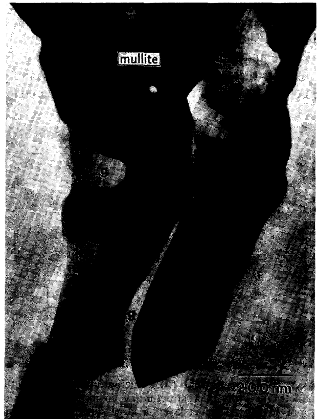
Fig. 6. Final stage in development of dendritic grain morphology in as-sprayed mullite, embedded in amorphous phase (labelled g).
