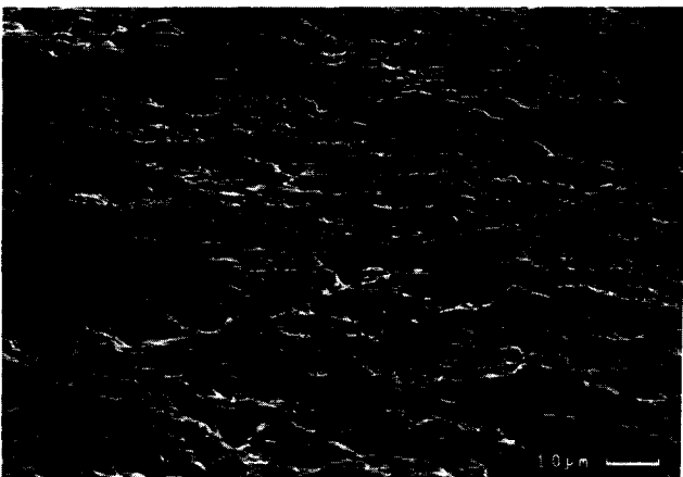
Fig. 9. A scanning electron micrograph of the edge of a disc of Z4.1 material after 6 h wear.
