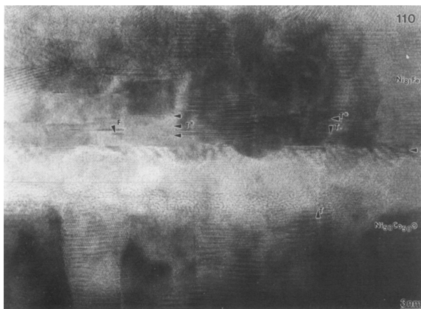
Fig. 26. Cross-section of NiO/CoO and Fe/Ni interface which is very rough, resulting in poor magnetic coupling (courtesy W. Cao).
