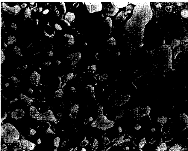
Fig. 1. Microphotographs of the structure of mullite-zirconia showing the scattering of zirconia particles.
