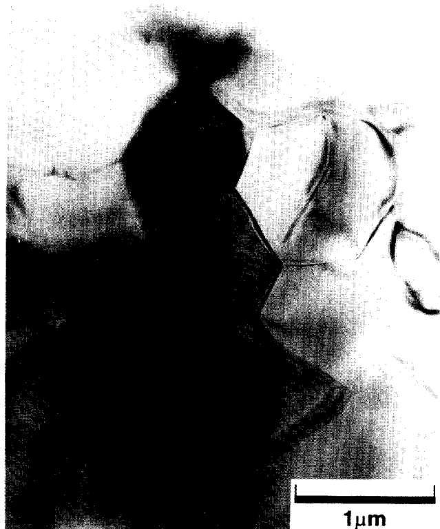
Fig. 9. TEM photograph showing granular-shaped mullite grains in the matrix of composites hot-pressed at 1650°C.
